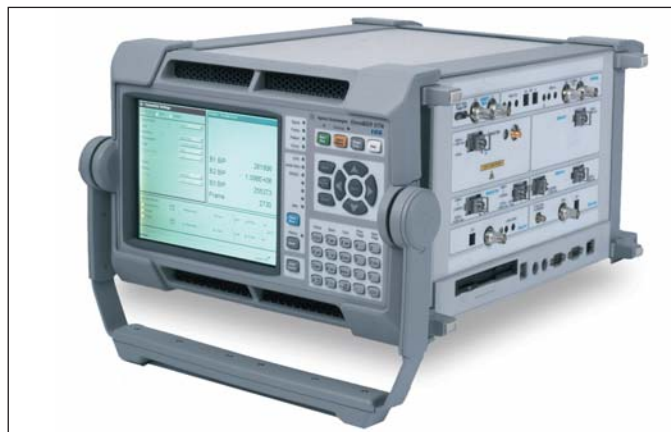
Figure 3 · Testing instruments such as Agilent's OmniBER OTN provide both a source of sinusoidal jitter and a method to assess BER in a single enclosure (depicted here on the instrument's screen).
