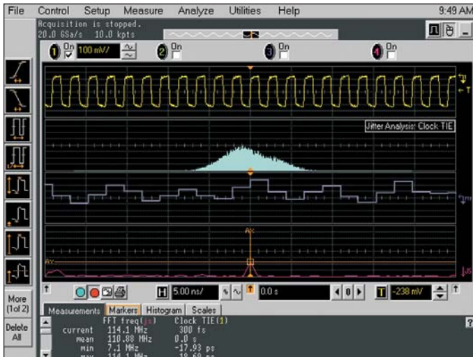
Figure 1 · High-speed, real-time digital storage oscilloscopes can display a number of views of the same signal. Shown here are a number of views of the 456 MHz clock signal at (A): a histogram of a transition point (B), TIE vs. time (C), and an FFT of the TIE data (D).
